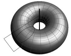
Interestingly, the volume  $2\pi^2 Rr^2$  of  $\tilde{\Omega}$  is equal to the area  $\pi r^2$  of  $\Omega$  multiplied by the distance  $2\pi R$  traveled by the center of  $\Omega$ . (Thus, it is also equal to the volume of the cylinder  $\{(x, y, z) : (x, z) \in \Omega, y \in [0, 2\pi R]\}$ . Moreover, this is a special case of a general property of all solids of revolution.
